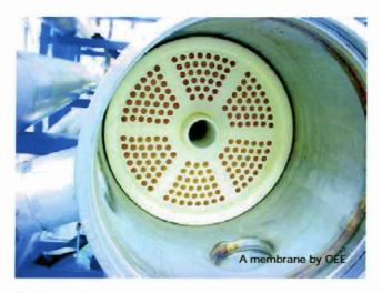
An integral part of desalination equipment consists of its membranes which have to perfectly suit the liquid separation processes. Each membrane is a specific filter which lets some water flow through while retaining dissolved minerals.
